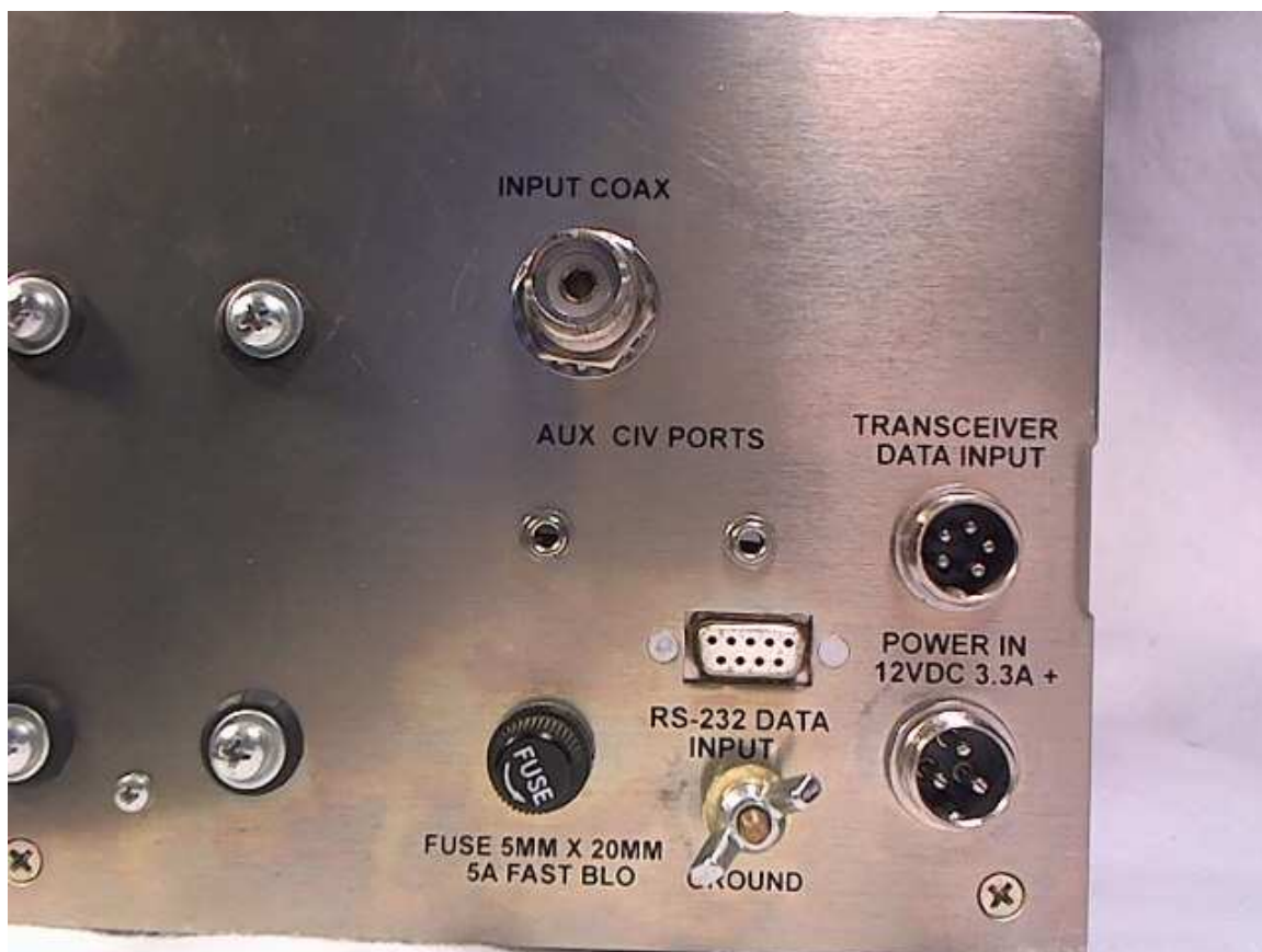
Figure 1.2: AT-AUTO (tm) Rear Panel prior to QRO Keyline Jack installation
