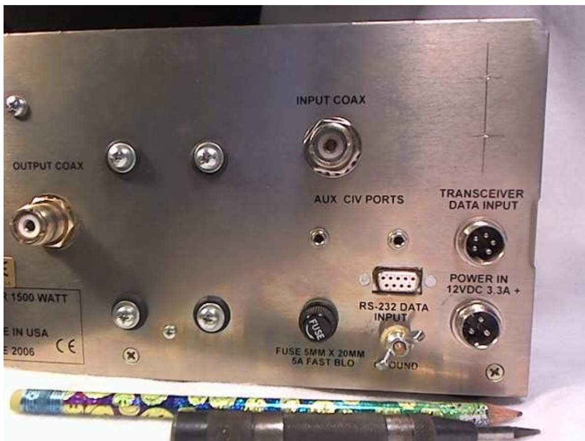
Figure 1.4: AT-AUTO (tm) Rear Panel showing intended QRO Keyline (RCA) jack locations
