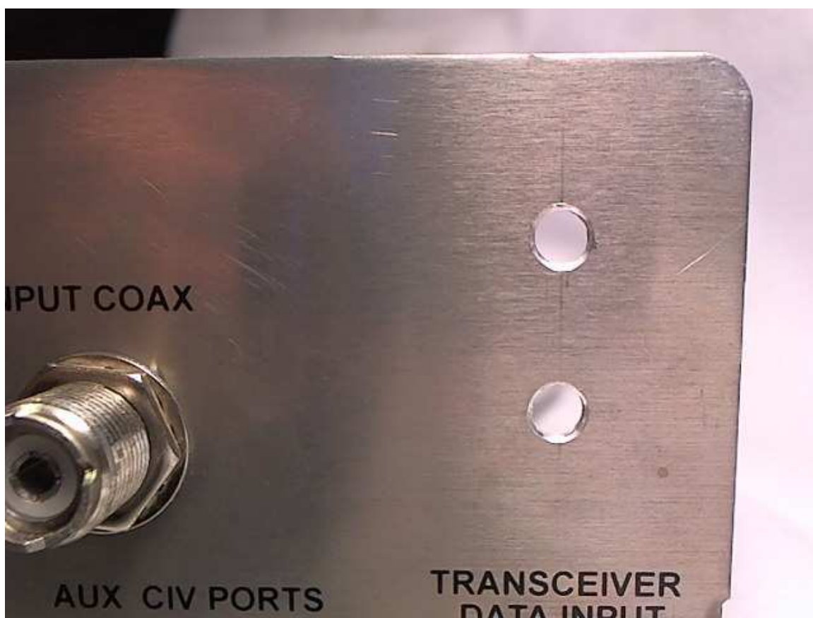
Figure 1.5: AT-AUTO (tm) Rear Panel with two holes added for RCA jacks
